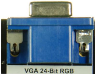
Figure 1. VGA output connector.
